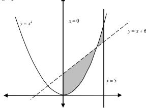
In this case it is very important to draw the graph, since the functions intersect between the boundaries. This means that we will have to actually calculate two separate integrals and then add the results. Otherwise we would end up subtracting the two pieces from each other.
